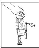
While holding a container over the uncapped VALVE to prevent splashing, turn water supply on and off a few times. Leave water supply off.
