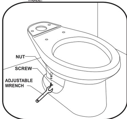
**2** REMOVE TOILET SEAT FROM ITS BOX AND PLACE IT IN NORMAL POSITION ON THE CLOSET FLANGE, WITH THE SCREWS INSIDE ITS BASE; BE SURE IT STANDS STRAIGHT. NEXT, PLACE THE NUTS AND SECURE THEM WELL WITH AN ADJUSTABLE WRENCH.
