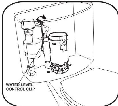
**14** TO CONTROL WATER LEVEL IN TANK, TAKE BOLT AND TURN IT COUNTERCLOCKWISE TO DECREASE WATER LEVEL AND CLOCKWISE TO INCREASE IT. **IMPORTANT:** Water level should be exactly as marked in the drain valve's overflow tube in order to flush properly.
