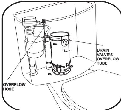
**6** TAKE OVERFLOW TUBE AND THE BASE TO FIX THE OVERFLOW TUBE; INSERT ONE END ON THE INTAKE VALVE TUBE AND THE OTHER END ON THE DRAIN VALVE'S OVERFLOW TUBE.
