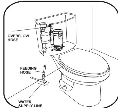
**7** TO SUPPLY WATER TO THE TOILET USE A FEEDING HOSE, WHICH HAS TO BE CONNECTED TO THE WATER SUPPLY LINE IN THE FLOOR.
